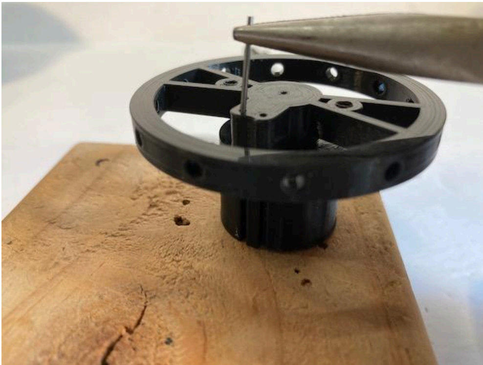
Insert and press 16 mm pins in the balance wheel
