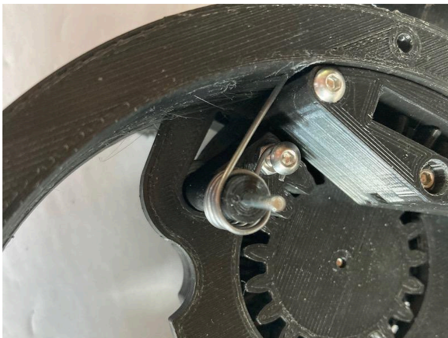
Ratchet in place with the 40 mm pin Notice the pin for the gear pushed below the surface of gear
