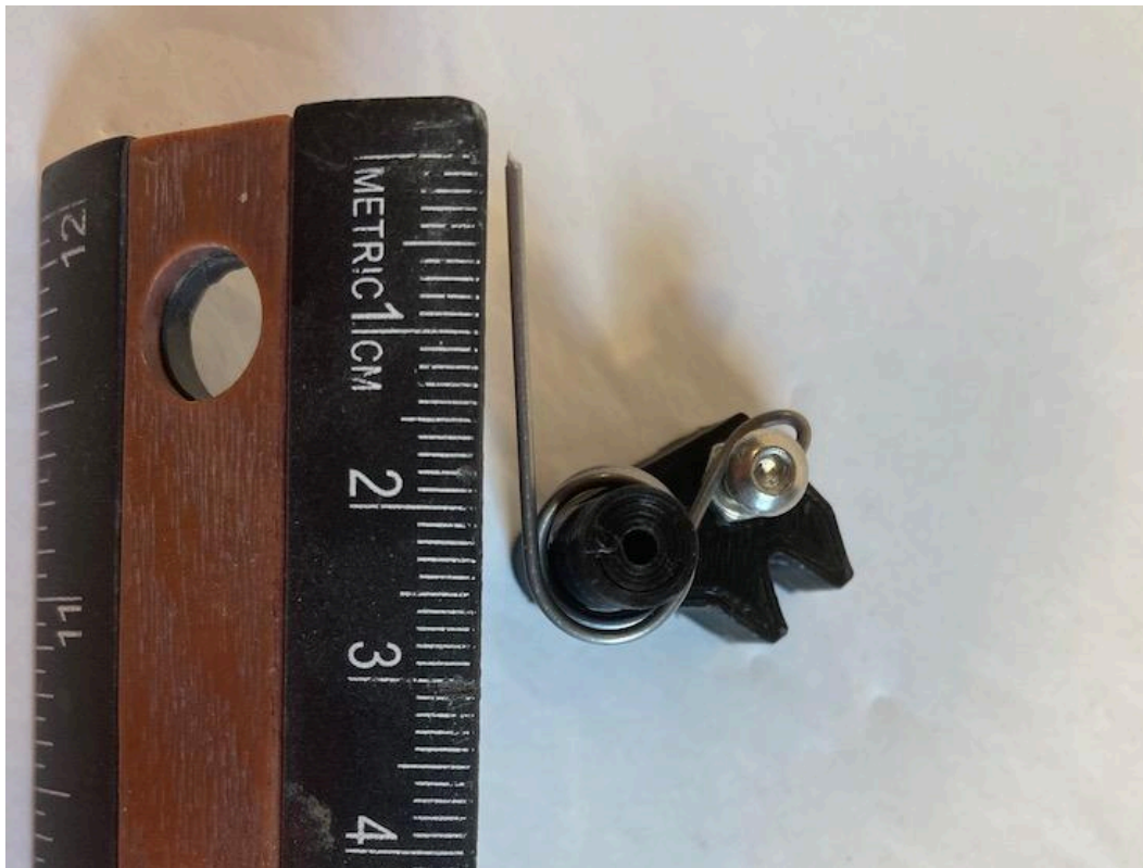
Ratchet in place with the 40 mm pin Notice the pin for the gear pushed below the surface of gear
