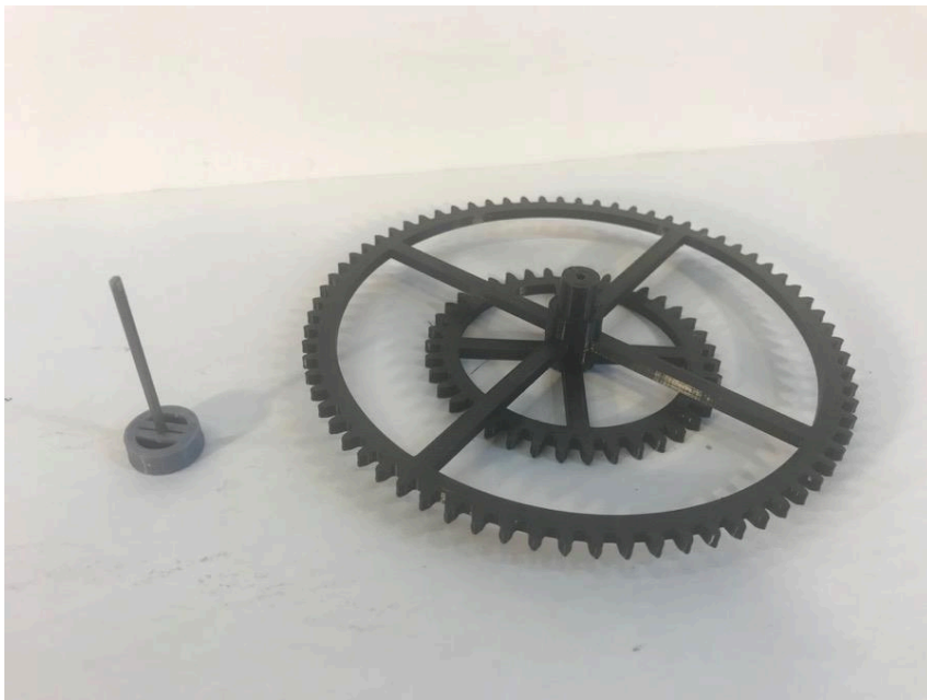
Install knob on 38 mm shaft
