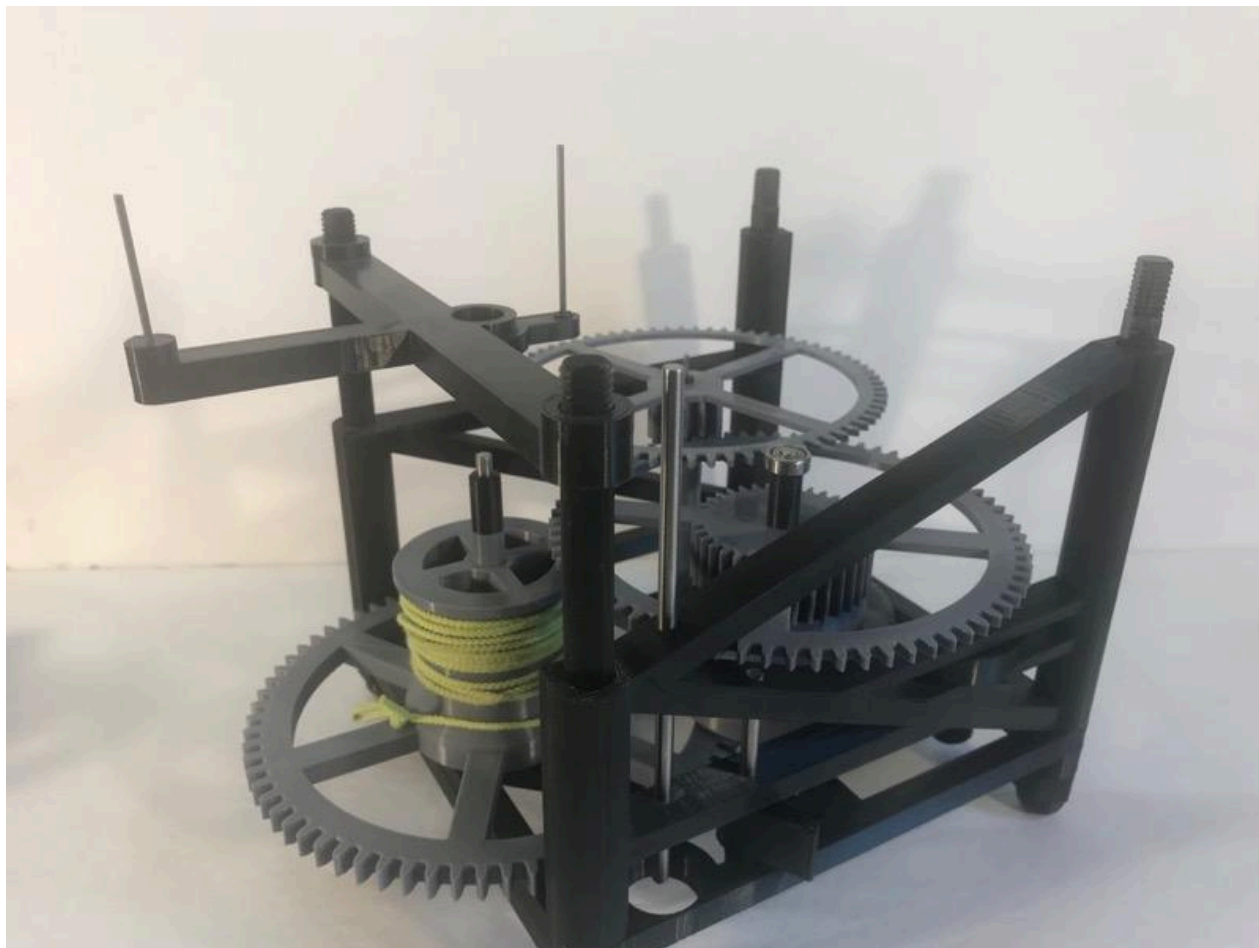
Install front escapement frame
