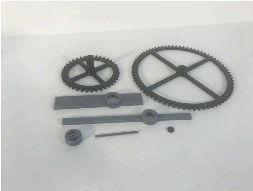
All parts, hour and minute gear and hands, 38 mm rod, knob
