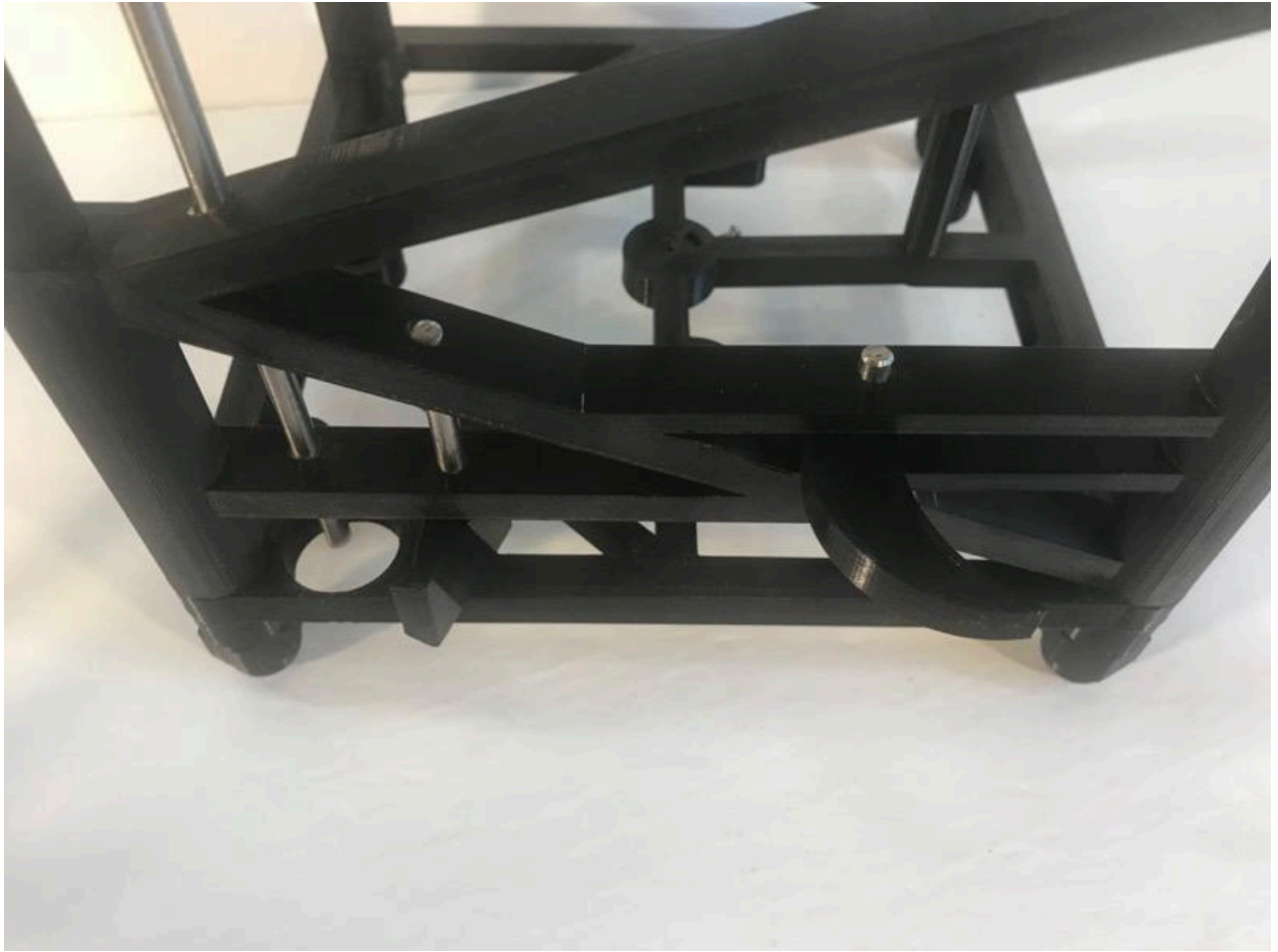
View on rewind stop and maintain ratchet
