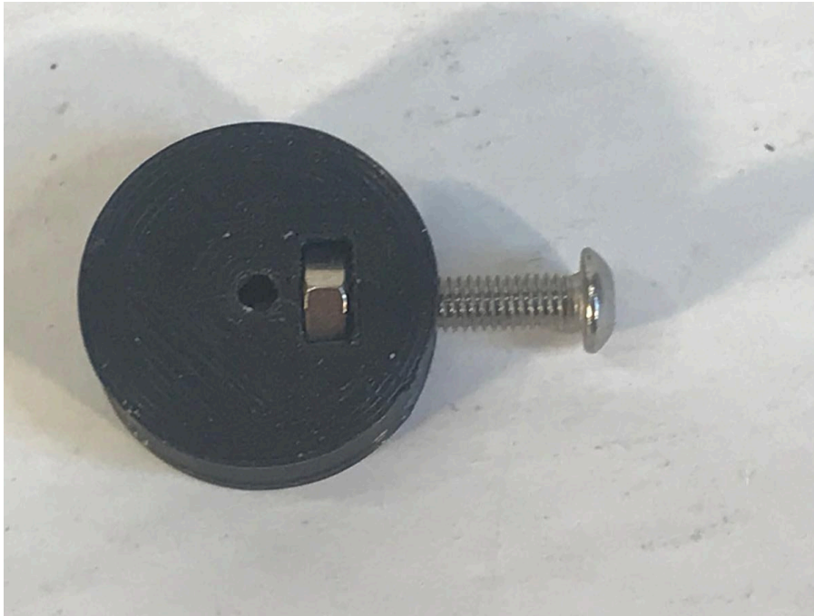
Ring, M3 x 12 screw and nut
