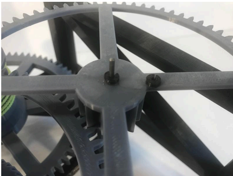
Add a 2 mm washer on top of gear
