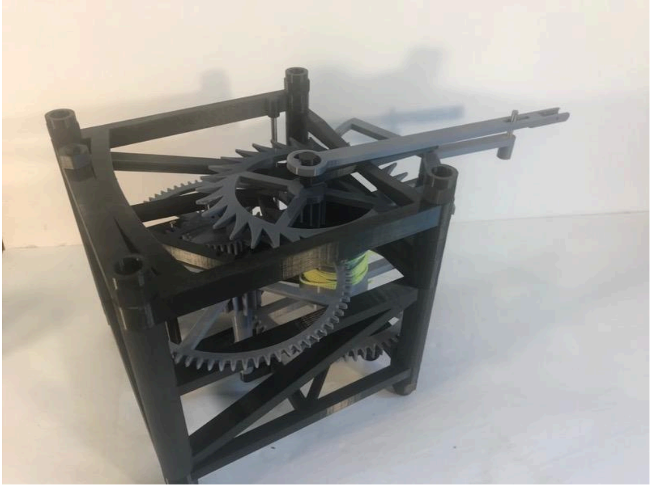
Check fit of pendulum crutch
